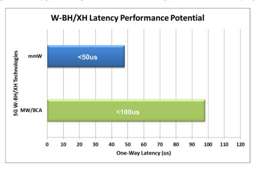
Figure 10: MW Backhaul/X-Haul Technologies Future Latency Performance
