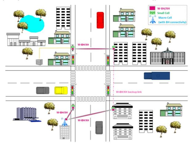
Figure 7: Small-Cell Backhaul/X-Haul Network Topologies
