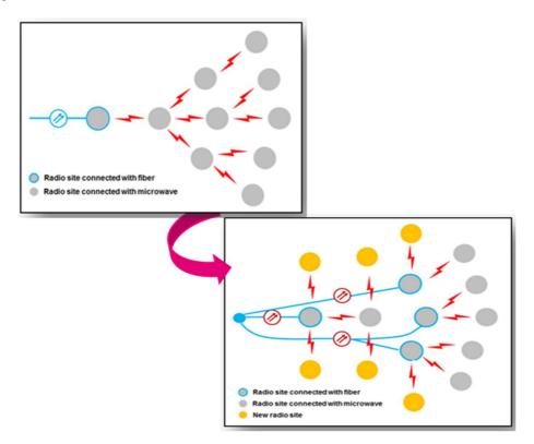
Figure 6: Macro-Cell Backhaul Network Topologies Shift
