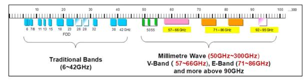
Figure 8: Microwave and Millimetre Wave Spectrum
