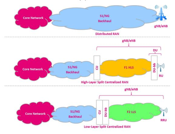
Figure 5: Distributed and Centralized RAN Architectures
