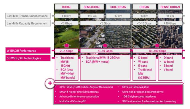
Figure 11: Wireless Backhaul/X-Haul Technologies Fit 5G
